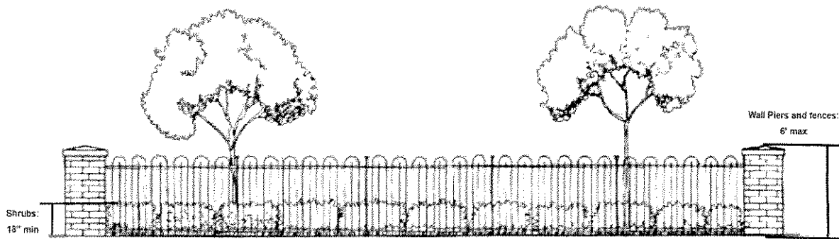
Figure C: A example of decorative pillar/wrought iron fence combination and shrub/tree line
