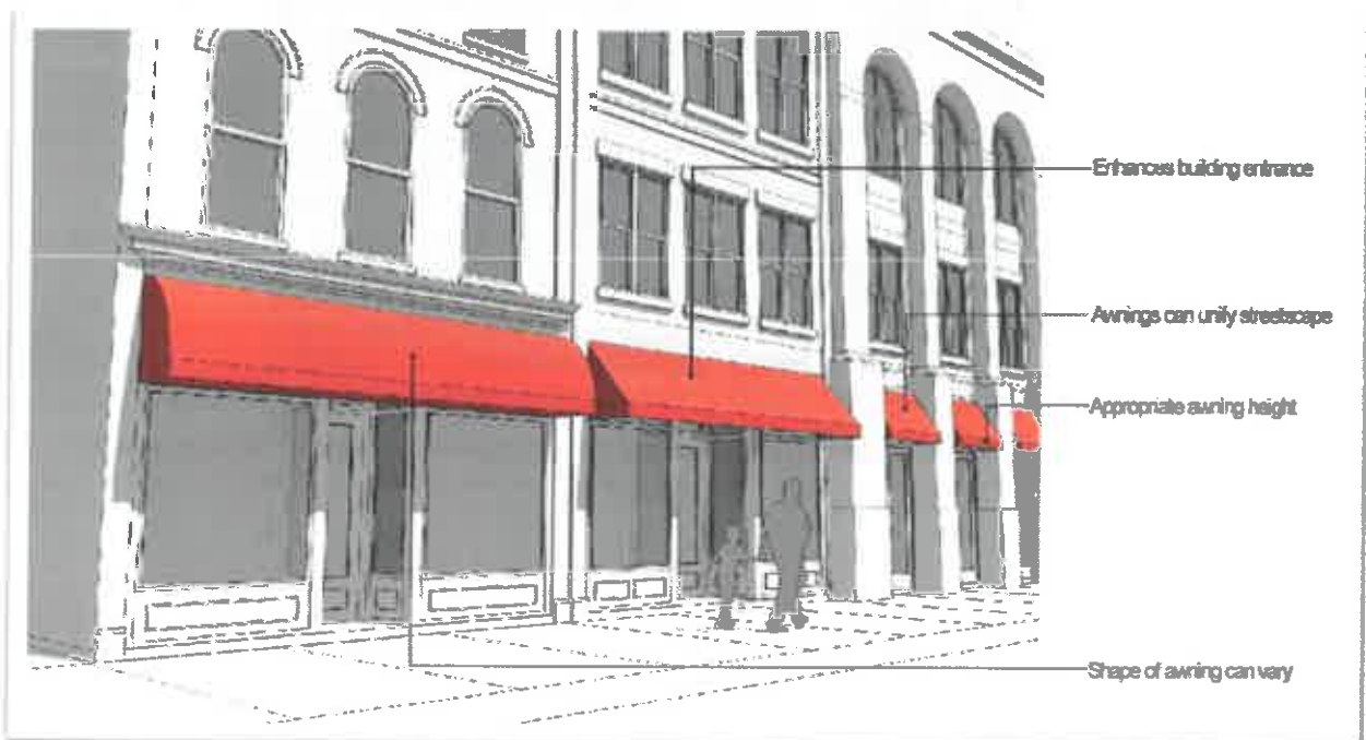
Figure 2.19: Encouraged Awnings —Awnings that do not obscure structural details, are simple in design, and are compatible with the building materials.
