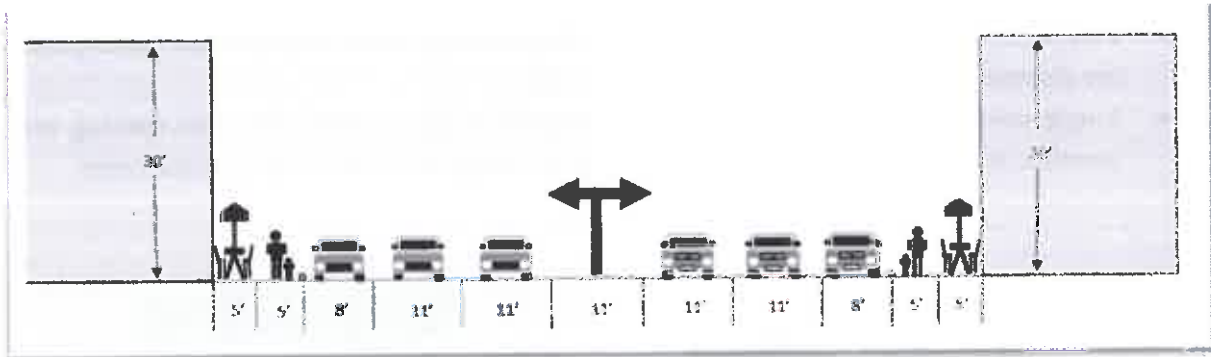
Figure 2.03 Building height, street width ratio: This illustrates a good design criterion that is the street width to building height ratio (1:3 Building heights to street width). Maintaining this ratio helps create the urban sense of enclosure.
