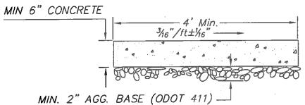
Sidewalk shall be constructed with a transverse slope of 3/16" per foot  $\pm 1/16$ ".
