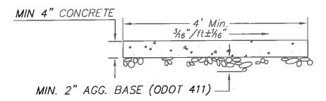
Sidewalk shall be constructed with a transverse slope of 3/16" per foot  $\pm 1/16$ ".
