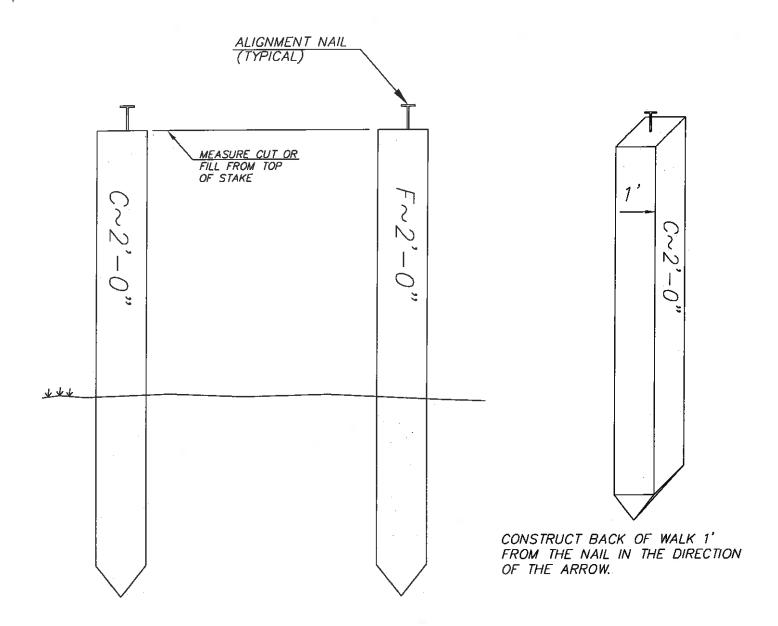
CUT 2'-0" FROM THE TOP OF THE STAKE (NOT THE ALIGNMENT NAIL) TO THE FINISHED GRADE OF THE WALK. FILL 2'-0" FROM THE TOP OF THE STAKE (NOT THE ALIGNMENT NAIL) TO THE FINISHED GRADE OF THE WALK.
