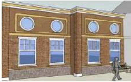
Figure 1161.2 - 1 Vertical Articulation Demarcation
