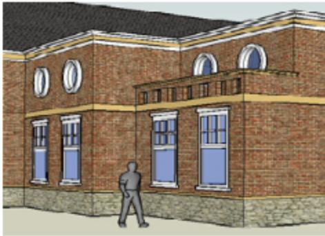
Figure 1161.2 - 1 Vertical Articulation - Recess
