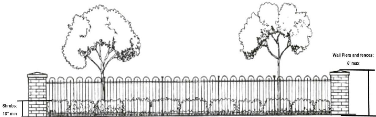
Figure C: An example of decorative pillar/wrought iron fence combination and shrub/tree line.
