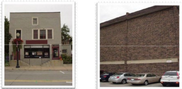
Figure 2.10 Discouraged Façade: These figures illustrate poor design through lack of detail, poorly spaced windows and doors, no sense of top, middle, and base, and minimal variation in materials and brick color.
